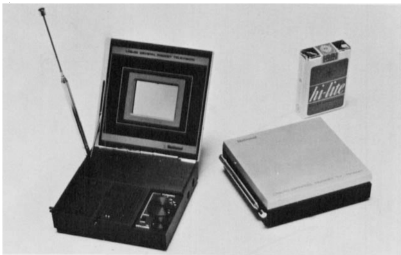
FIGURE 7 Developmental small liquid crystal television display.
